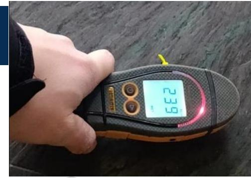
Elevated moisture readings indicating failed membrane allowing water to travel under front door.
